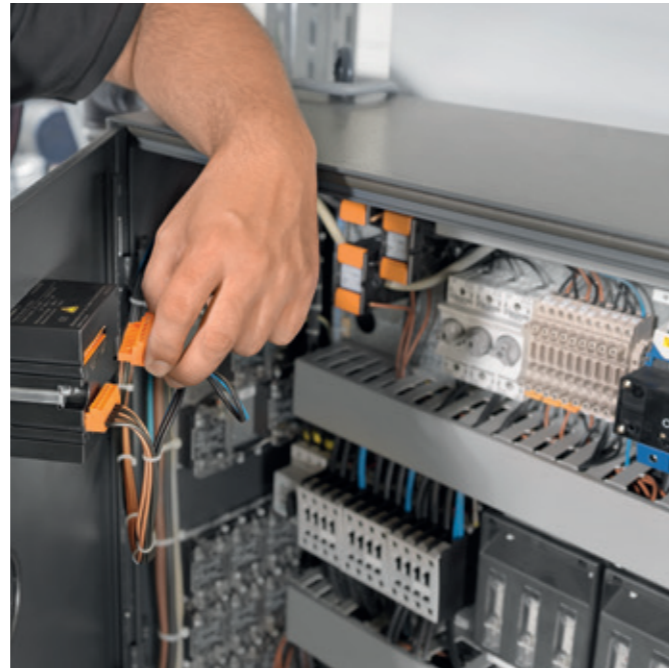
Efficient cable assembly for small and medium production batches, e. g. in panel building.
