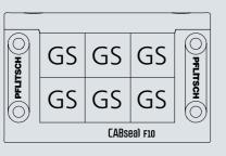
Assemble individually as you need it: With CABseal, all grommets can be freely positioned in the frames.
