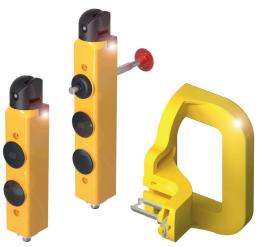
Safety switches with separate actuator are protection devices which simultaneously provide personal and machine protection. Together with a machine controller and a guard they secure the hazardous area against access. Depending on the requirements, safety switches without guard locking, with mechanical guard locking, or with electrical guard locking can be used.
