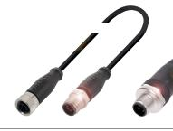
3 m cable PUR (black) with M12 female (straight), M12 male (straight), 4-pin
