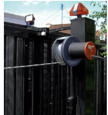
Slip ring assembly in gate locking system
