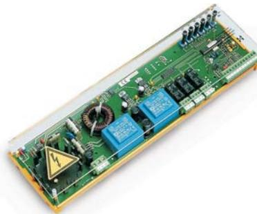
The ESG is typically used for controlling single-phase capacitor start motors in a variety of systems. Applications include heating, ventilation and pumping systems. The ESG can also be used for the control of lighting systems. In heating and ventilation systems, Pt1000's are used to measure the temperature to regulate output levels (motor speed) and switch-points are controlled according to the levels set by potentiometers.
