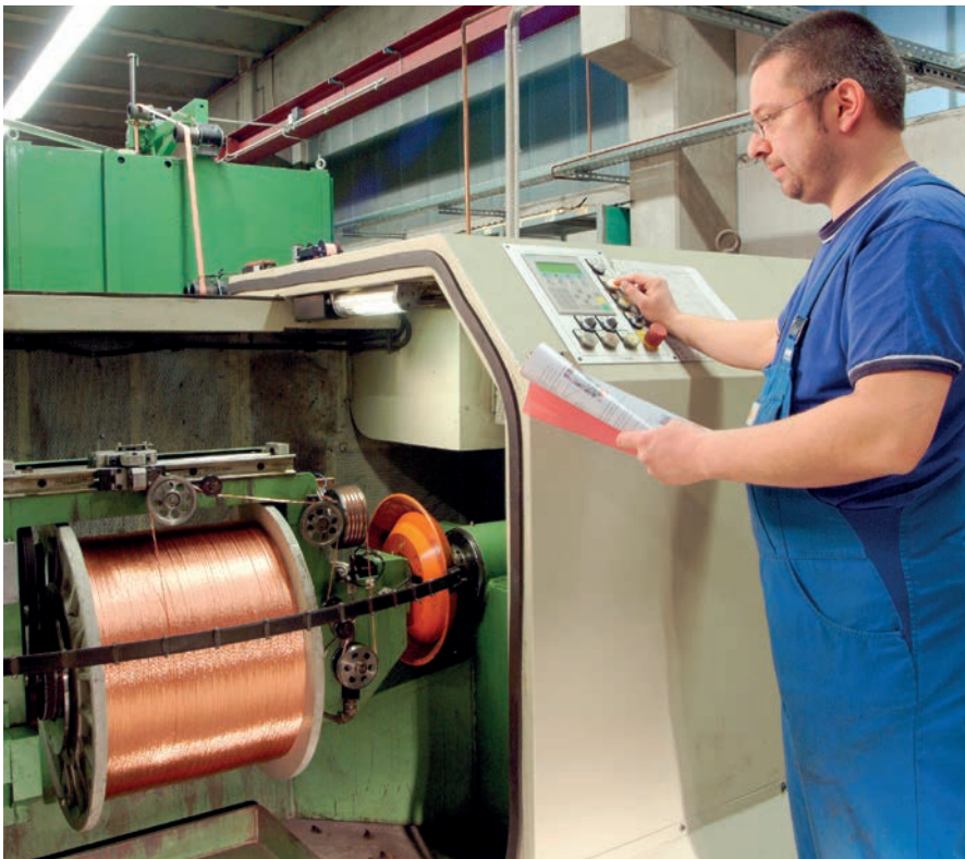
Twisting and stranding of highly flexible conductors
