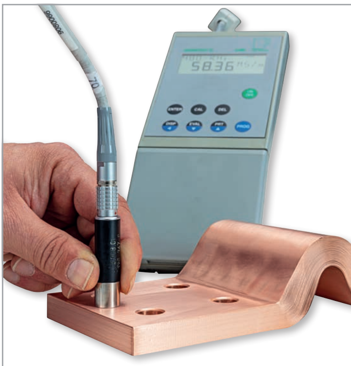
Conductivity test/flexible foil-connectors
