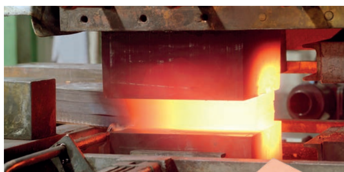
Pressure welding process for copper connectors
