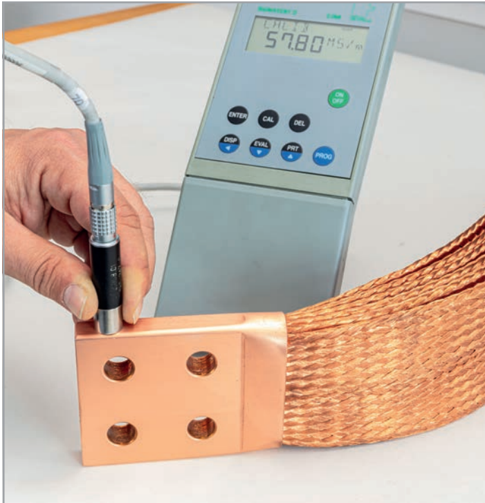
Conductivity test/flexible braided connectors
