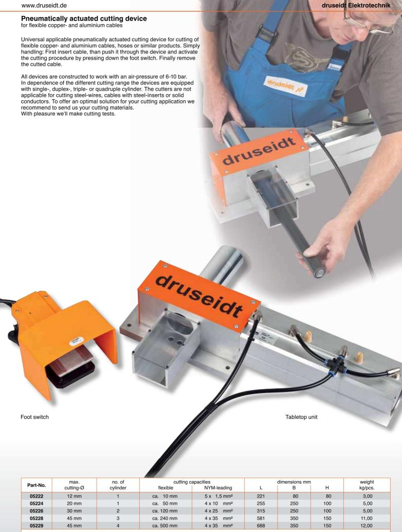
**Remark:** The specified cutting capacities in the table are only circa values. They are in dependence of the hardness and thickness of the insulating material as well as of the cable stranding. All values in the table are identified by an air pressure of 8 bar.
