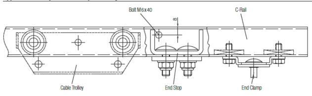
The end stop is fixed in the C-rail between the end clamp and the cable trolley.
